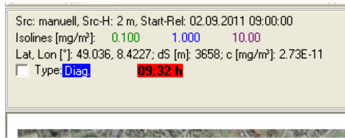
Fig. 4.4: Information Bar during an accidental release calculation
