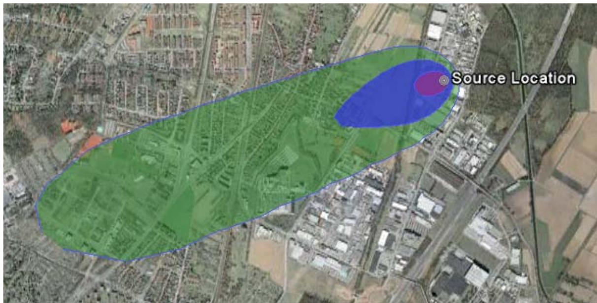
Fig. 4.3: Three isolines of pollutant concentration
