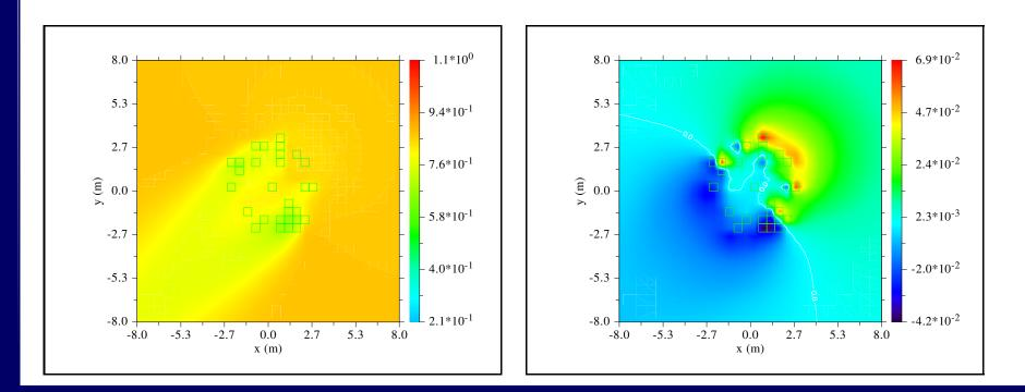
Turbulent kinetic energy (m<sup>2</sup>/s<sup>2</sup>, left) and turbulent energy dissipation (m<sup>2</sup>/s<sup>3</sup>, right), horizontal cross-section at z = 5.25 m
