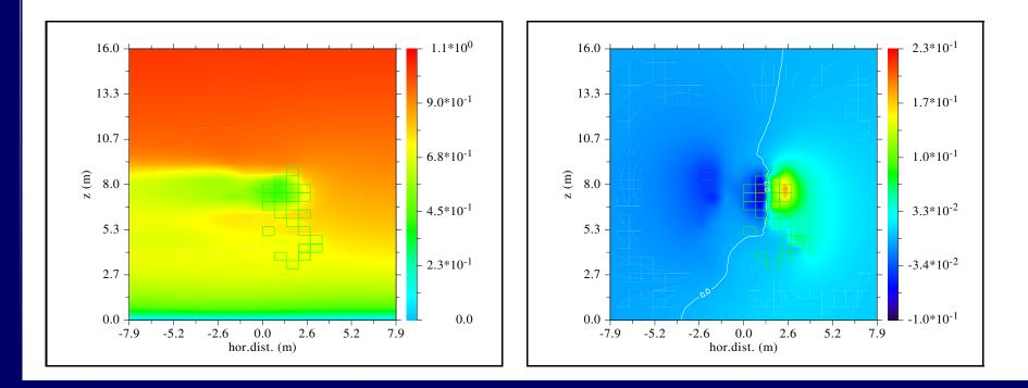
Turbulent kinetic energy ( $m^2/s^2$ , left) and turbulent energy dissipation ( $m^2/s^3$ , right), vertical cross-section SW — NE
